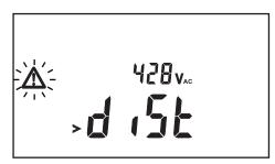
The spurious voltage present on the terminals is too high for a measurement to be made:
