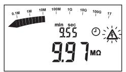
Start the measurement by a long press on the START/STOP key. The long press is acknowledged by an audible beep.
