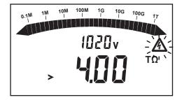
The insulation resistance is outside the measurement range.
