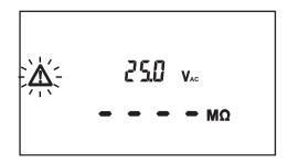
The spurious voltage present on the terminals is greater than 25 VAC or 35 Vpeak.
