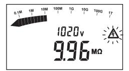
During measurements the instrument will beep every 10 seconds to alert the user that a high voltage is present.
