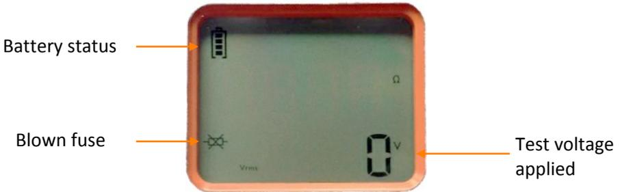
\*LCD is shown indicating a blown fuse.
